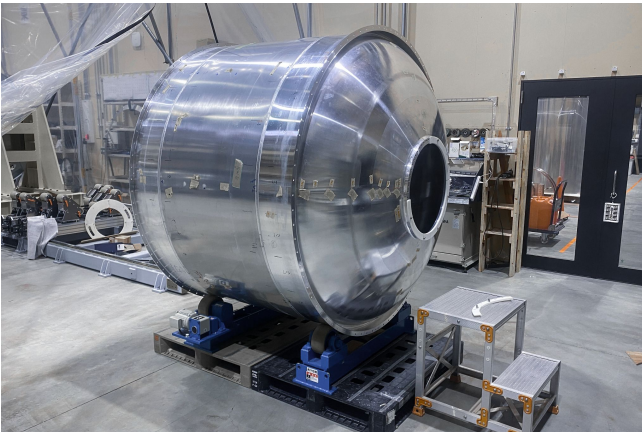
Second Stage Propellant Tank with Completed Welding
